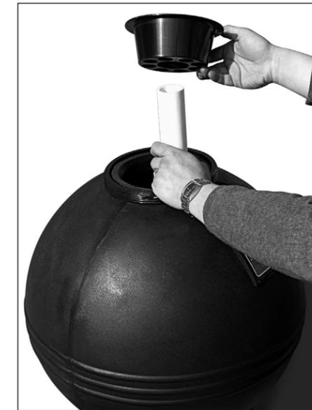
2. Turn filter over. Place next to pool between skimmer and return opening on pool. Place sand filter over stand pipe. *Add approximately 3 inches of water before adding sand.* Add required #20 grade silica sand: See sand chart on back page. Remove sand fill guide and save.
