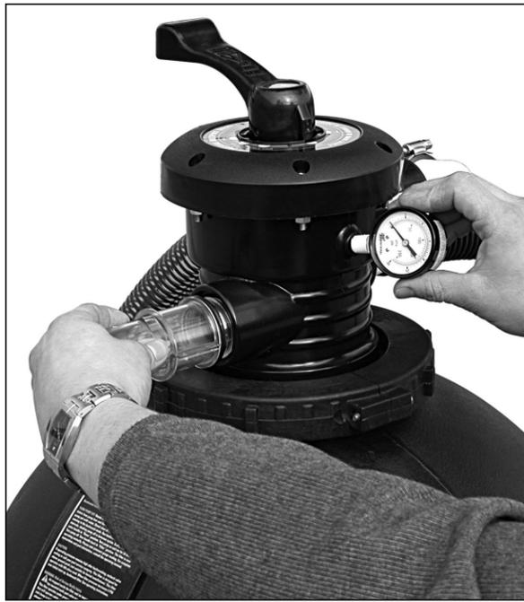
13. Apply Teflon tape to threads of pressure gauge (4 wraps ideal) and thread into valve. Install waste adapter by pushing O-ring over threads of clear adapter and threading into waste port.
