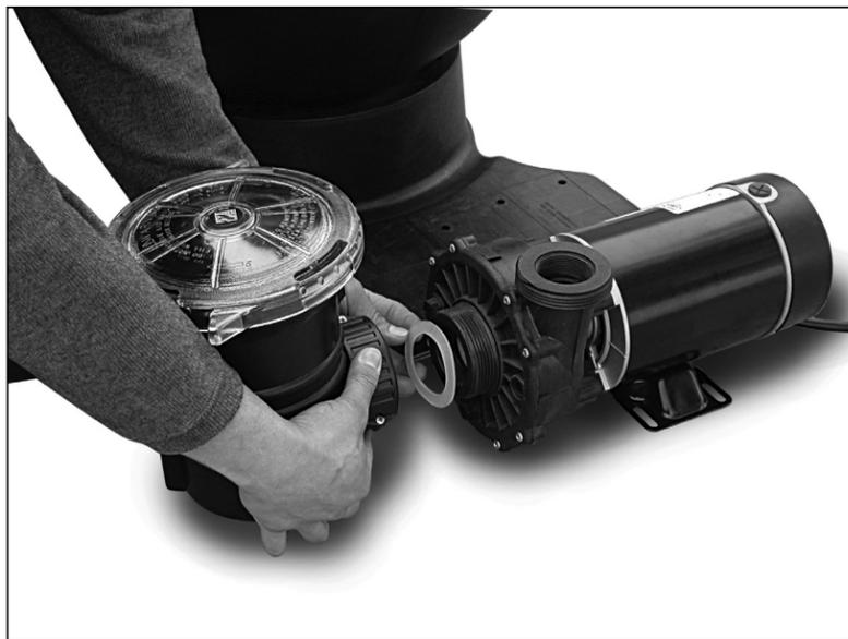
7. Install trap base to pump by removing gasket from inside trap. Remove clear trap lid, and place gasket in trap nut. Thread onto pump, **DO NOT OVER-TIGHTEN**. Place pump with trap onto pump base. Remember to replace trap lid.
