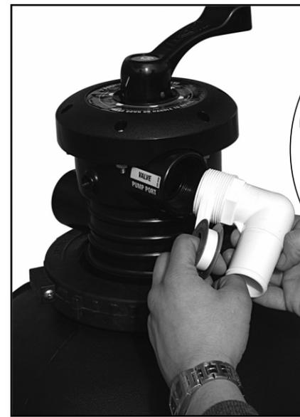
9. Apply Teflon tape to smooth 90° hose adapter threads (4 wraps) and thread into valve pump port.
