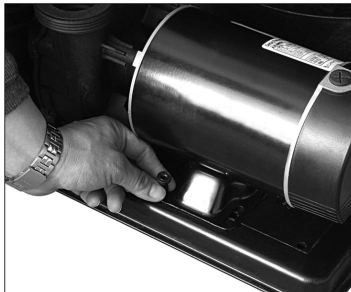
8. Install anchors into slots of pump into holes in pump base. Push pins into anchors to secure.
