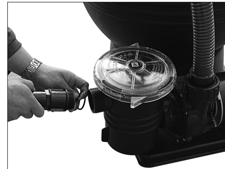
12. Put O-ring over thread on 1 1/2" smooth straight hose adapter and thread into front of pump basket.
