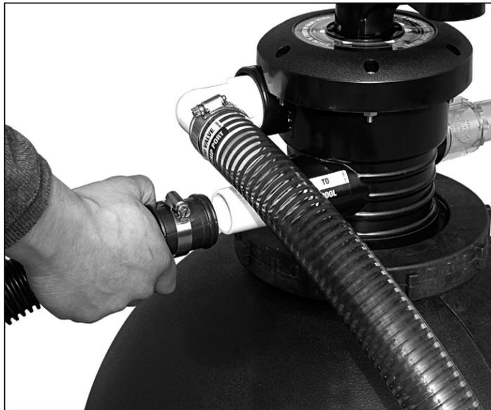
15. Install hose onto smooth hose adapter in valve by loosening hose clamp and sliding over adapter end. Install other end onto return fitting of pool and tighten clamps.
