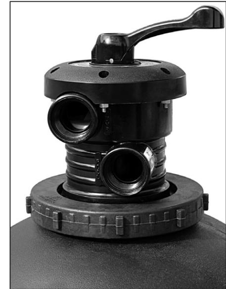
6. Split-nut is fully installed when threads on body are not exposed. Retighten bolt on split-nut.
